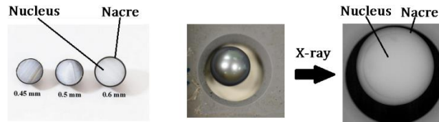
Fig. 1. A cut through three Tahitian pearls (left), a Tahitian pearl positioned in a borehole of a wooden plate for X-raying (middle) and the resulting X-ray image (right).
