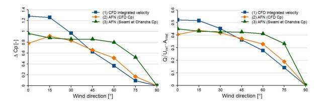
Figure 2: Wind pressure coefficient difference and non-dimensional airflow rate as a function of wind direction – results based on CFD simulation for the cubic building case
